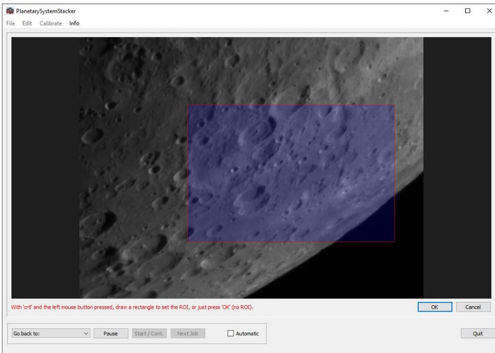
Optionally, stacking can be restricted to a so-called region of interest (ROI) smaller than the intersection of all frames. To specify its size a viewer opens and prompts the user to select the ROI as a rectangular patch (as described in Section 4.8 above). Selecting the full view instead of a ROI is accomplished by just pressing "OK".
