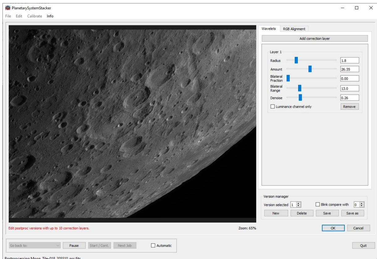
Sharpening in PSS is implemented as a multi-layer wavelet scheme. For each processing version a different hierarchy of correction layers with increasing filter radius values can be defined. In the basic pa-
