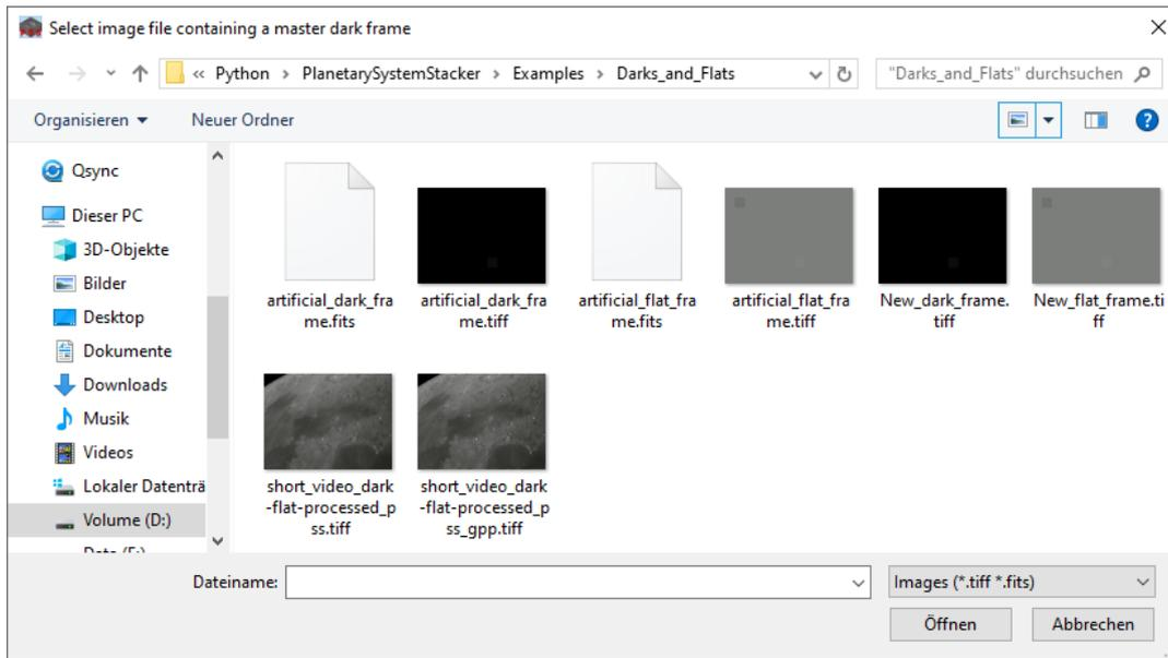
Calibration in PSS can be done using either dark frame or flat frame correction, or both. In the latter case, make sure to create the master dark frame first. This way it is used already when the master flat frame is processed.
