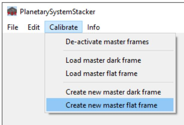
First the dark / flat input videos (or directories with still images) have to be processed into so-called “master frames”. To do so, select the menu entry “Create new master dark frame” or “Create new master flat frame” from the “Calibrate” menu. When the file chooser opens, select the input video or directory.
