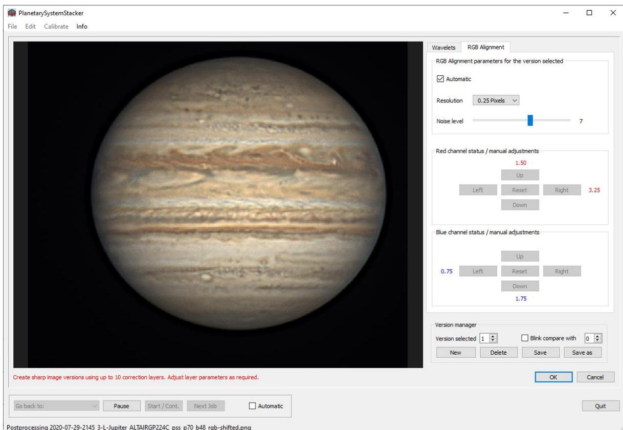
The red and blue figures in the channel status panels show the shifts applied to the red and blue channel in pixels.
