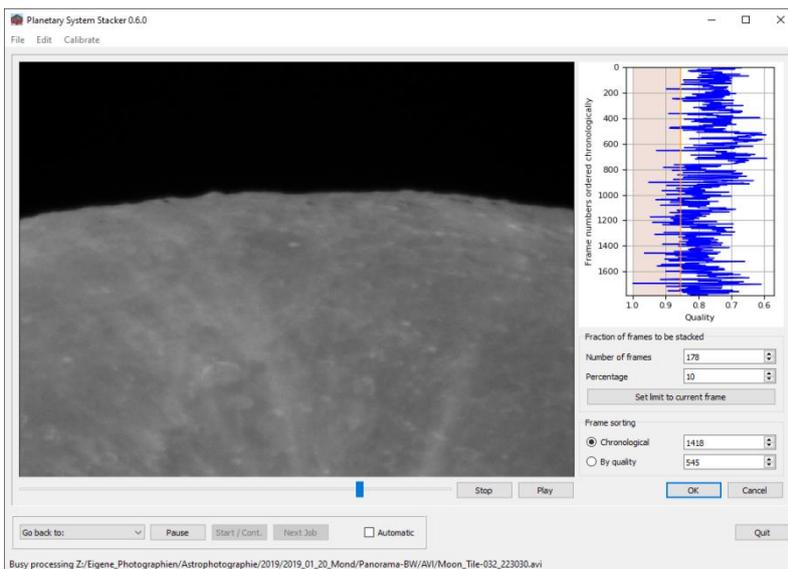
By setting the "Frame ordering" checkbox, frames can be ordered either by quality or chronologically. In the latter case, as demonstrated to the left, the quality graph usually is quite busy, as a consequence of rapid quality variations caused by seeing.
