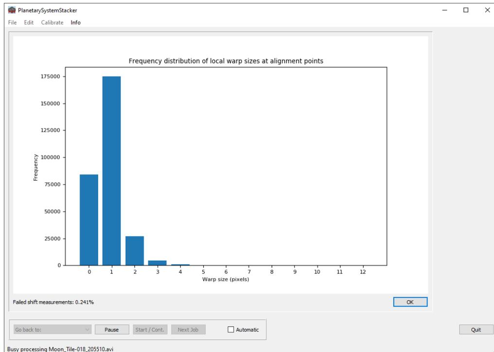
Another quality indicator for the warp shift compensation is the fraction of failed shift measurements which is displayed below the shift distribution graph. If this value is above 5%, it is written in red color. In this case it is a good idea to experiment with different parameter settings, as discussed above. A high value, however, not necessarily means that the results are bad. Other explanations are a very low contrast in the image, or oversampling in the optics / camera configuration.
