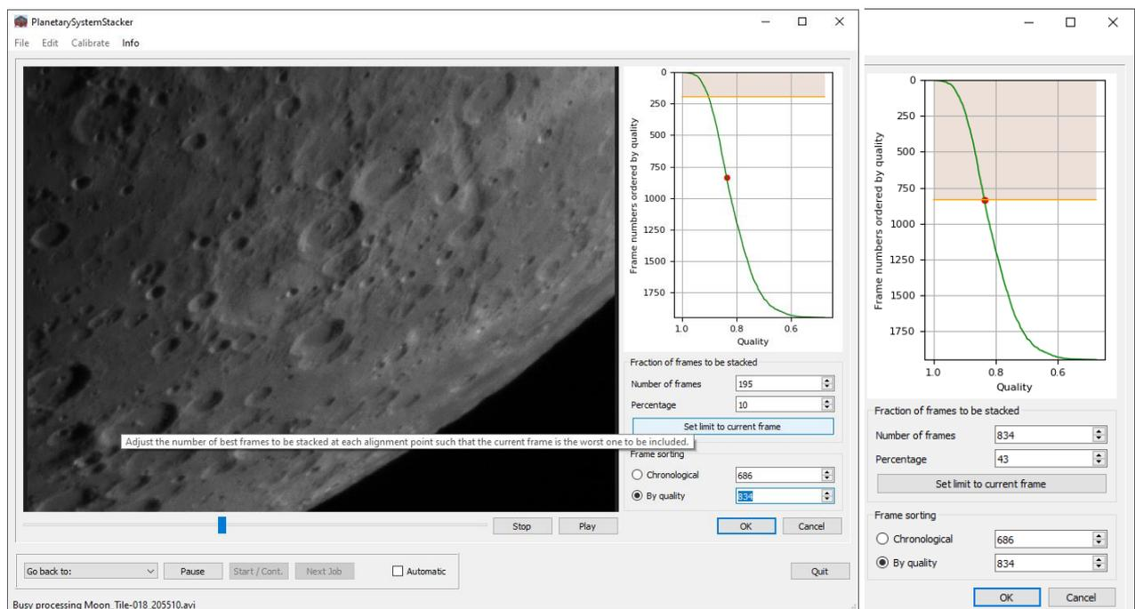
In the next step the user decides how many frames are used for stacking. The GUI opens a view on the scene where frames can be displayed either ordered by decreasing overall quality or chronologically. With a horizontal slider the user can scroll through all frames. As an alternative, he or she can press "Play" / "Stop" to display frames as a video.
