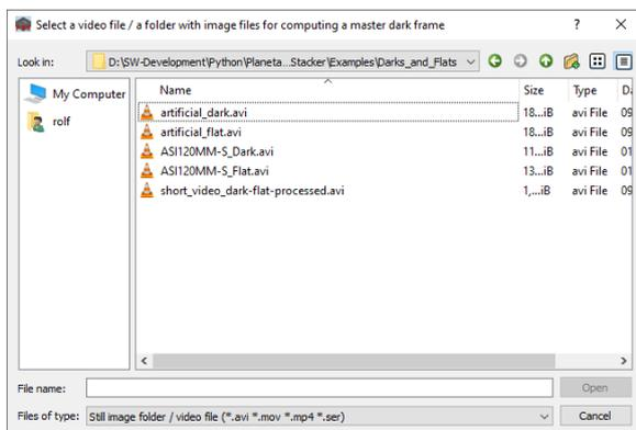
When the processing finishes, another file chooser opens to select the location where the master frame is to be stored as a 16bit .png (or .tiff or .fits) file. If you do not want to store the master frame, just press “cancel”. In this case the master frame is still kept in memory for image calibration during this PSS session.
