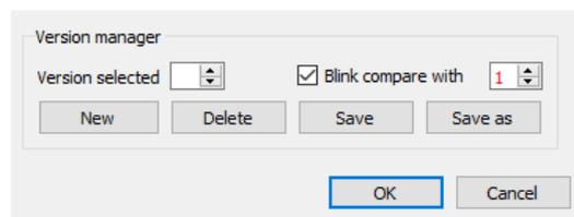
Once the user is satisfied with the selected version, pressing the "OK" button triggers PSS to save this image version along with the input image (as a 16bit .png, .tiff or .fits image). The file name is the one of the input image, extended by the suffix "\_gpp.png / .tiff / .fits". The parameters of all postprocessing
