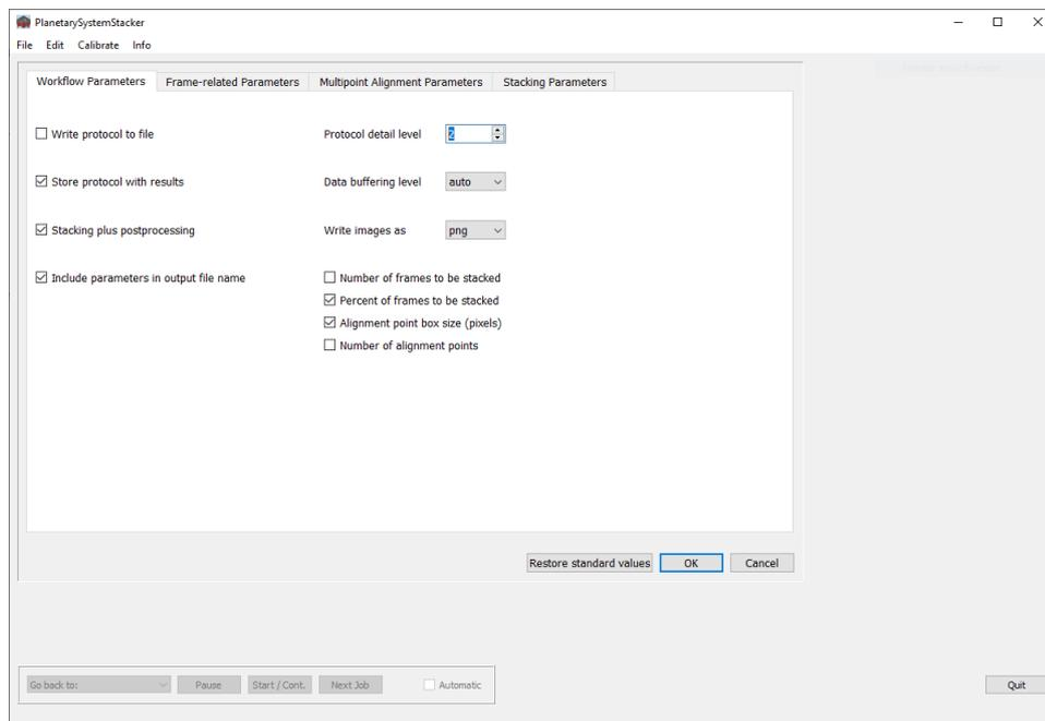
When the program is started for the first time, a view opens automatically for the input of individual parameters. The parameters are arranged in tabbed pane windows relating to workflow control, frame stabilization, multi-point alignment, and stacking.
