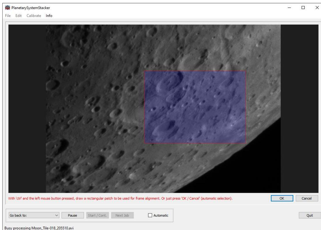
PSS offers to identify the stabilization anchor automatically (check "Automatic frame stabilization"). If this option is chosen, additional parameters ("patch size" and "search width") can be modified to control the automatic algorithm. Obviously, in batch mode automatic stabilization is the only choice, so the configuration parameter "Automatic frame stabilization" has no effect.
