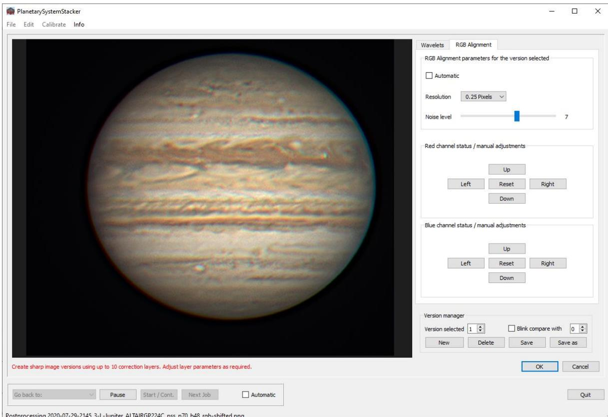
If, for example, the object was low in the sky during capturing, the three video color channels are misaligned due to differential atmospheric dispersion. As a result, color fringes appear at sharp edges such as
