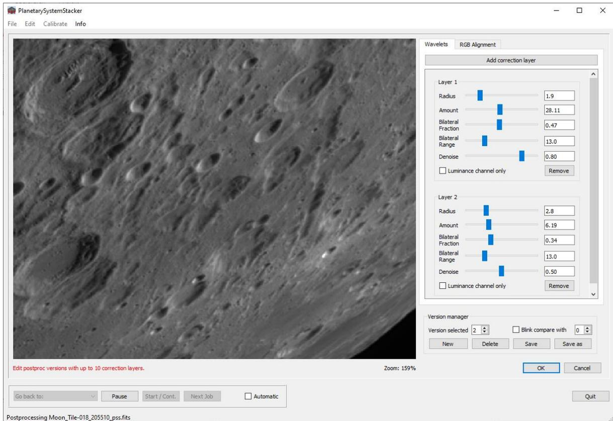
In the above example a second layer has been added, and bilateral filtering is used for both layers. The viewer's zoom function has been applied to look at the filter effect in detail. The current zoom rate is always shown at the lower right corner of the viewer. Pressing "1" resets the viewer to 100%.
